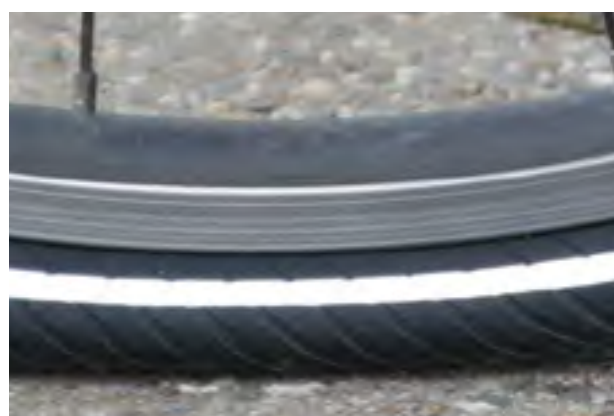
Illustration 93 : Pression largement insuffisante
