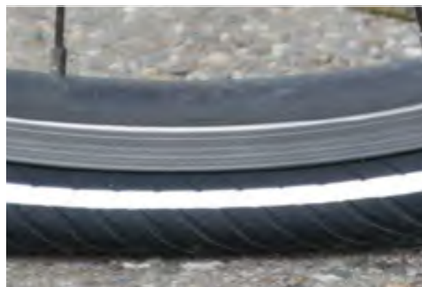
Illustration 87 : Pression largement insuffisante
