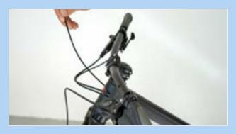
Figure 216: Attaching the end cap
