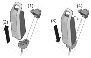
Figure 124: Removing and inserting the frame battery
