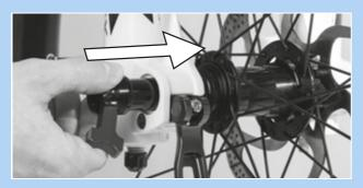
Figure 69: Inserting the cross axle in the direction of the arrow
