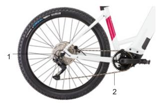
Figure 29: Chain drive with derailleur gears
