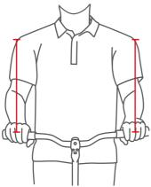
Figure 93: Determining the optimal handlebar width
