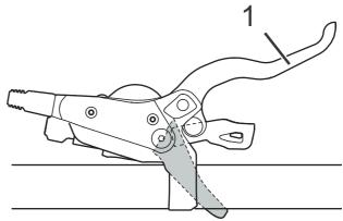
Figure 46: Front wheel (2) and rear (1) brake levers – Shimano brake used as an example
