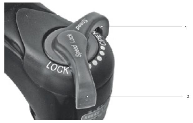
Figure 133: Suntour compression adjuster in open (1) and closed (2) position
