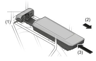
Figure 125: Removing (2) and inserting (3) the pannier rack battery
