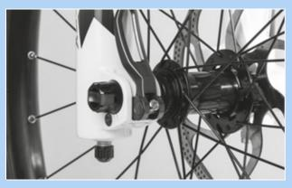
Figure 154: Adjusting the quick release clamping force
