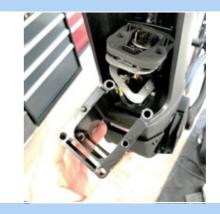
Figure 55: Pulling out the PowerTube adapter
