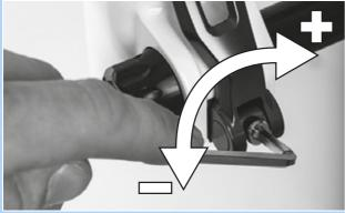
Figure 155: Adjusting the quick release clamping force
