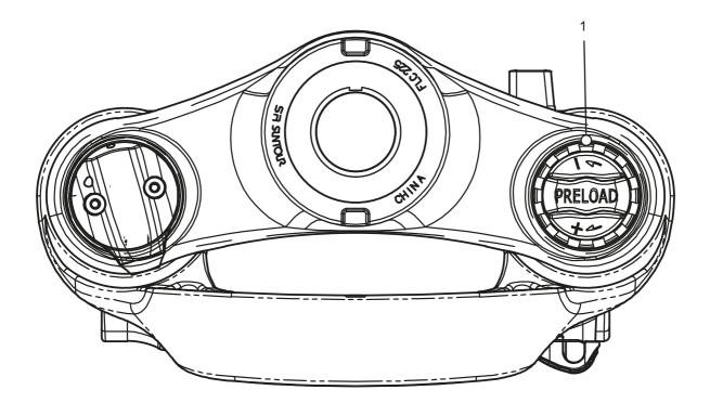
Figure 109: Sag setting wheel (1) on the suspension fork crown
