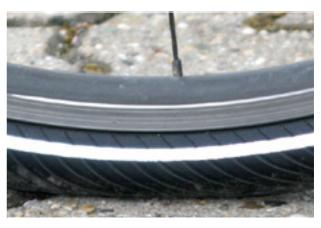
Figure 102: Correct tyre pressure. The tyre is barely deformed under the load of the body weight
