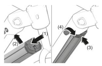
Figure 127: Inserting the integrated battery
