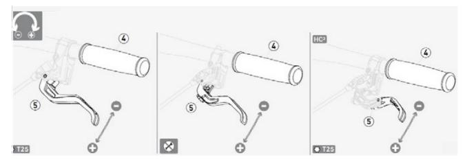
Figure 108: Adjusting the grip distance on a MAGURA disc brake lever
