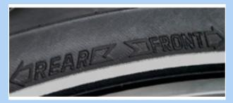
Figure 80: Rotation direction arrow on MTB tyres
