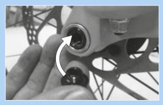
Figure 67: Pushing the quick release lever into the axle
