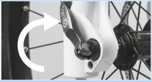
Figure 78: Closing the quick release
