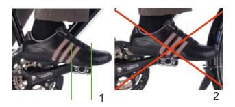
Figure 123: Correct (1) and incorrect (2) foot position on the pedal
