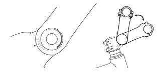
Figure 99: Different versions of angle-adjustable stems
