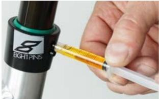
Figure 142: Lubricating the seat post tube
