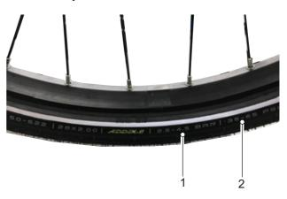
Figure 143: Tyre pressure in bar (1) and psi (2)
