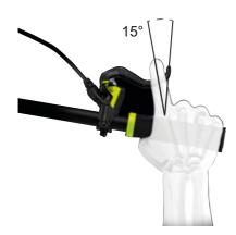
Figure 104: Brake handle position
