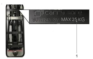
Figure 122: The maximum load bearing (1) capacity is indicated on the pannier rack.
