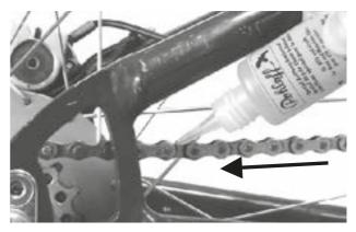
Figure 141: Lubricating the chain
