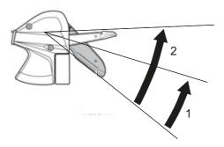
Figure 134: Switching gears with lever A, using gear shift SL-M315 as an example
