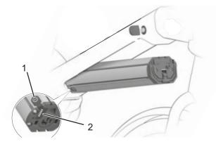
Figure 49: Position of charge level indicator on integrated battery
