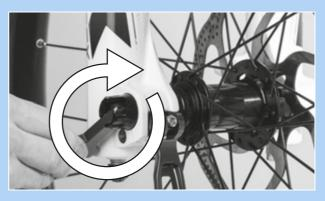
Figure 70: Tighten the axle in the direction of the arrow
