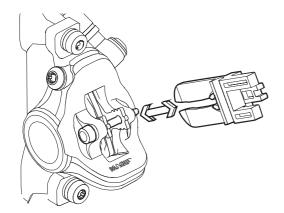
Figure 51: Fastening the transport securing device
