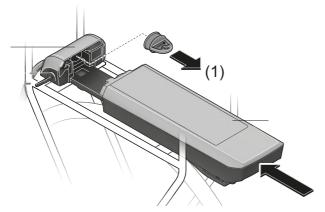
Figure 128: Covering open contacts with cover cap – example: pannier rack battery
