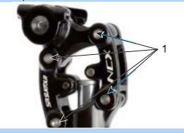
Figure 156: SR Suntour suspension seat post lubrication points
