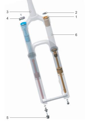
Figure 14: Internal structure of air suspension fork
