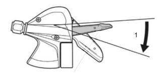
Figure 135: Switching gears with lever B, using gear shift SL-M315 as an example
