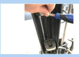
Figure 54: Removing hexagon screws
