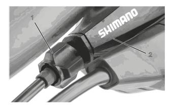
Figure 151: Adjusting sleeve (1) for the single-cable, Bowden--cable-operated gear shift with shifter housing (2), example
