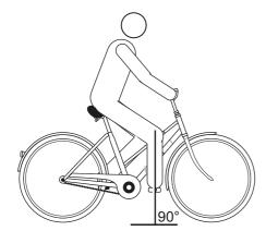
Figure 91: Knee cap perpendicular line
