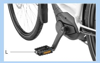
Figure 82: L-pedal in the left-hand crank arm
