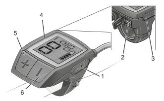
Figure 129: BOSCH Purion on-board computer layout
