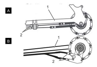
Figure 152: Adjusting sleeves (2) on two alternative versions (A and B) of a dual-cable, Bowden-cable-operated gear shift on the chain stay (1)
