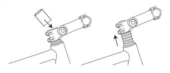
Figure 98: Raising the Ahead stem by fitting spacer rings
