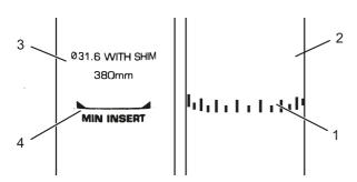
Figure 89: Detailed view of the seat post – examples of the minimum insertion depth marking
