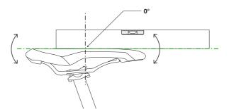
Figure 92: Horizontal saddle tilt with 0° tilt in the centre of the saddle
