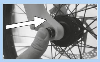
Figure 65: Inserting the axle in the direction of the arrow
