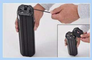
Figure 61: Detaching the upper interface
