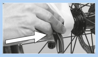
Figure 76: Inserting the quick release in the direction of the arrow
