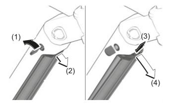
Figure 126: Removing the integrated battery
