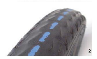
Figure 144: Tyre without tread which can still be used (1) and tyre with puncture protection showing through (2), which needs to be replaced
