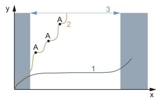
Figure 140: Diagram showing wear, operating hours (x) vs. material erosion (y)
