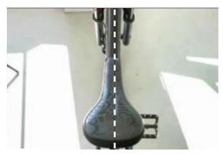
Figure 85: Positioning the saddle in direction of travel
