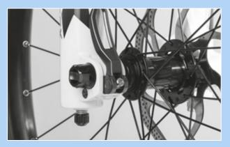
Figure 73: Perfect position for the clamping lever
