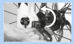
Figure 72: Pressing the quick release lever in the direction of the arrow
