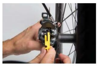
Figure 146: Checking the brake lining when fitted with the help of the transport safety wear gauge
