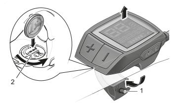
Figure 130: On-board computer with attachment screw (1) and battery compartment cover (2)
