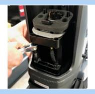
Figure 53: Removing the 4 mm hexagon screws
