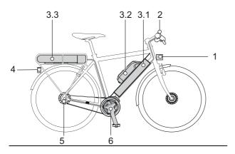
Figure 31: Diagram of an electric drive system with electric components
