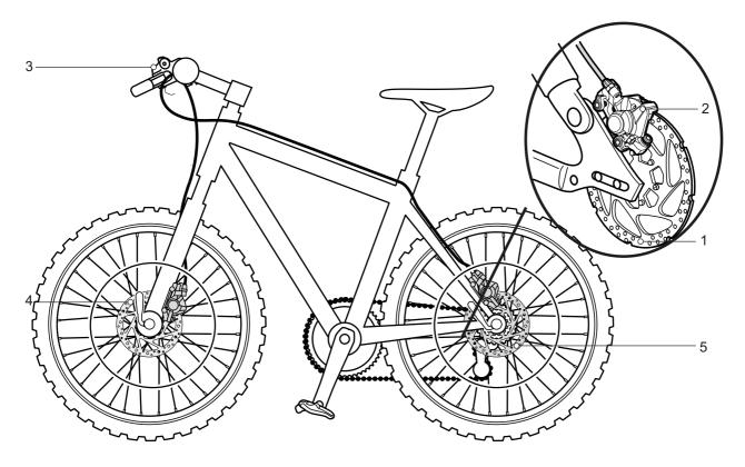
Figure 22: Brake system with disc brake – example
