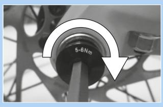
Figure 68: Tightening the securing screw
