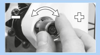
Figure 77: Adjusting the clamping
