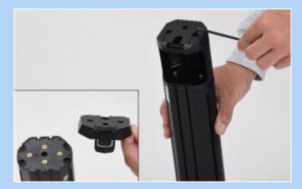
Figure 63: Fastening the battery mounting plate
