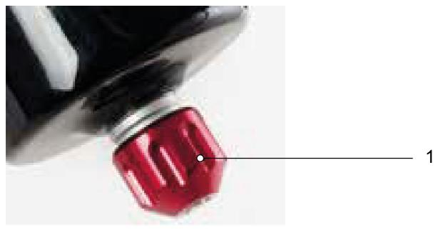
Figure 112: Example of Suntour rebound screw (1)
