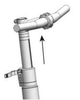
Figure 96: Pulling the locking lever upwards; All Up used as an example
