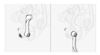
Figure 24: Rim brake locking lever closed (1) and open (2)
