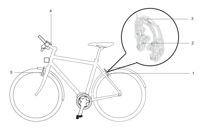
Figure 23: Brake system with rim brake in detail - MAGURA HS22 used as an example
