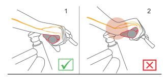
Figure 101: Correct (1) and incorrect (2) position of the handle
