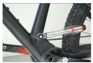
Figure 86: Tightening the seat post axle
