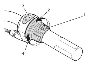
Figure 136: Example: use of SHIMANO Nexus gear shift
