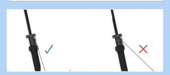
Figure 163: Bowden cable position
