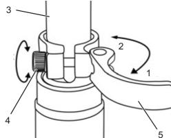
Figure 88: Opening the seat post quick release
