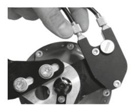
Figure 150: The tension adjuster on Rohloff hub versions with external switch control is located on the cable box positioned on the left-hand side
