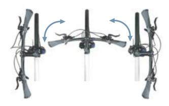
Figure 4: Twist function, using BY.SCHULZ as an example
