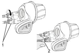
Figure 153: Twist grip with adjusting sleeves (1) and play in the gear shift (2)  $% \left( 2\right) =2$
