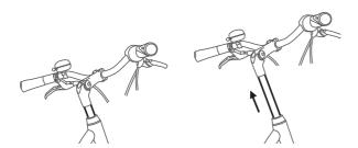
Figure 97: Adjusting the quill stem height
