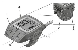
Figure 116: BOSCH Purion on-board computer layout
