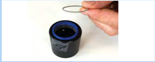
Figure 151: Removed spring washer
