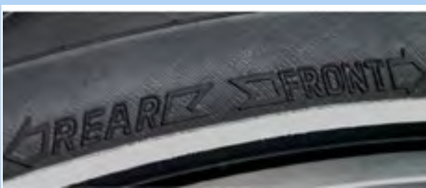
Figure 50: Rotation direction arrow on MTB tyres
