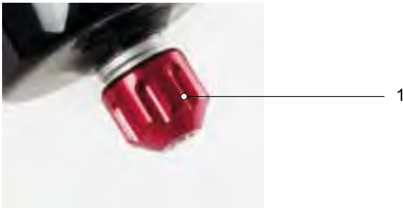
Figure 207: Suntour rebound screw (1)
