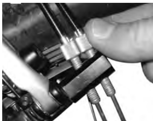
Figure 134: The tension adjuster on Rohloff hub versions with internal switch control is located on the tension counter support
