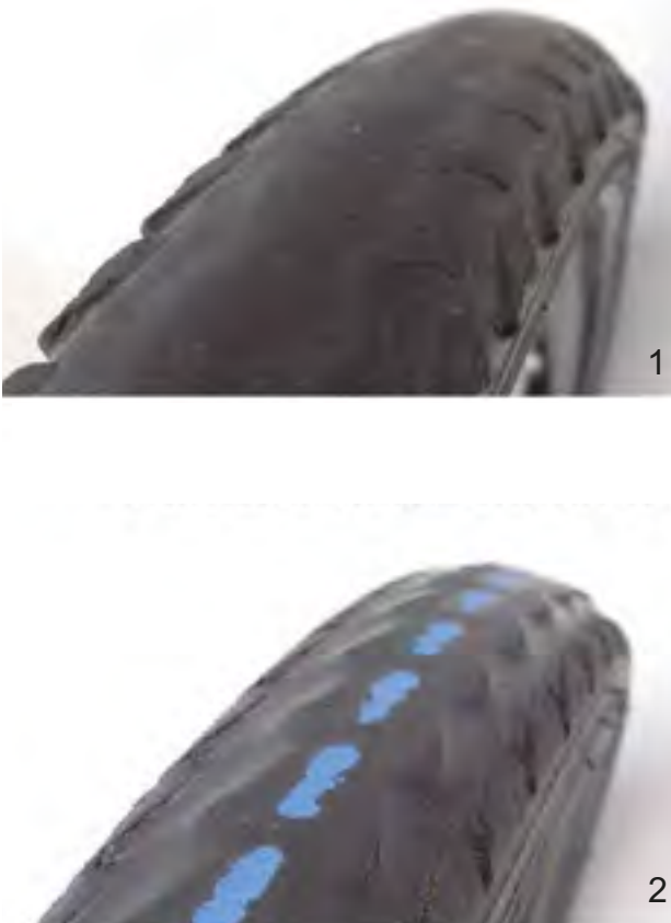
Figure 129: Tyre without tread which can still be used (1) and tyre with puncture protection showing through (2), which needs to be replaced
