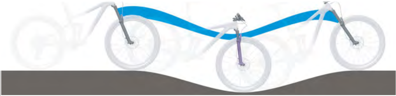
Figure 208: Excessively soft suspension in the suspension fork on hilly terrain
