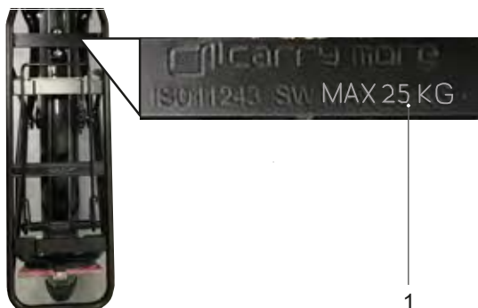
Figure 107: The maximum load bearing (1) capacity is indicated on the pannier rack.
