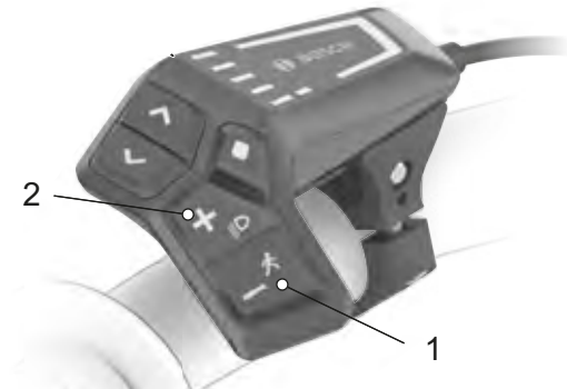
Figure 116: Position of plus and minus buttons
