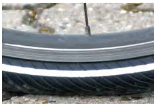
Figure 92: Correct tyre pressure. The tyre is barely deformed under the load of the body weight
