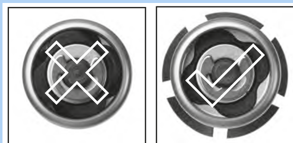
Figure 61: Closed and opened flange
