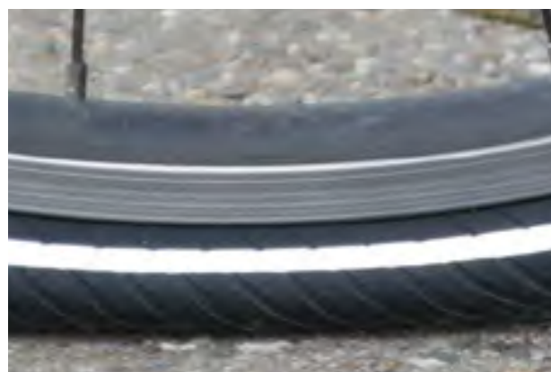
Figure 93: Much too little tyre pressure
