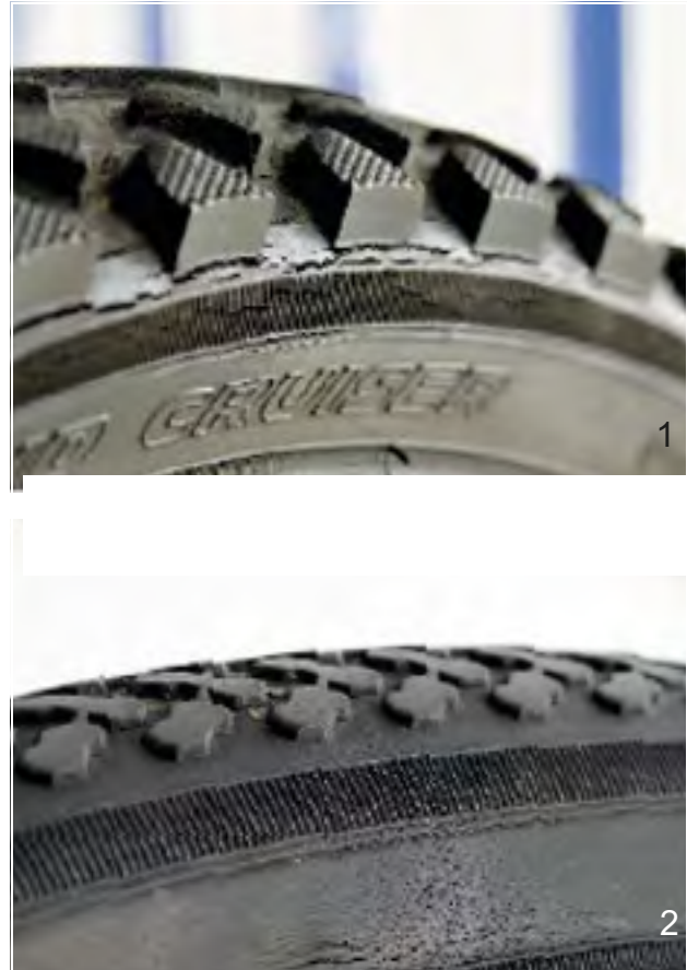
Figure 130: Examples of fatigue cracks (1) and ageing cracks (2)
