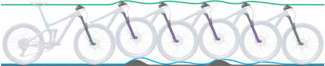
Figure 204: Suspension fork rebounding too quickly
