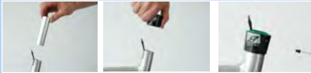
Figure 166: Fitting the slide bushing and outer sleeve
