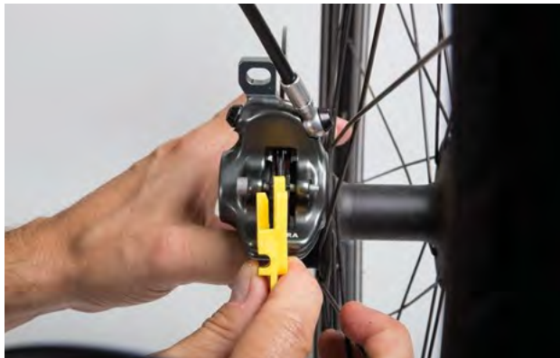
Figure 131: Checking the brake lining when fitted with the help of the transport safety wear gauge
