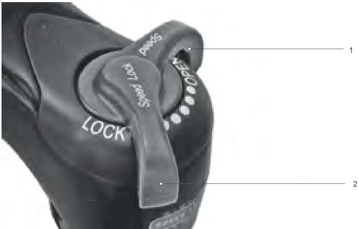
Figure 121: Suntour compression adjuster in open (1) and closed (2) position
