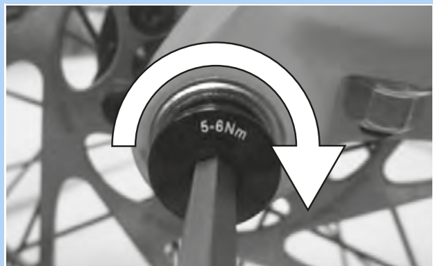
Figure 54: Tightening the securing screw
