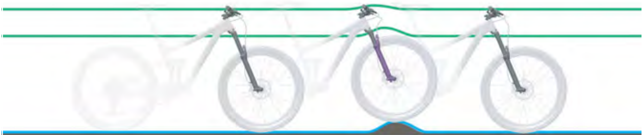
Figure 10: Optimum fork riding performance over bumps
