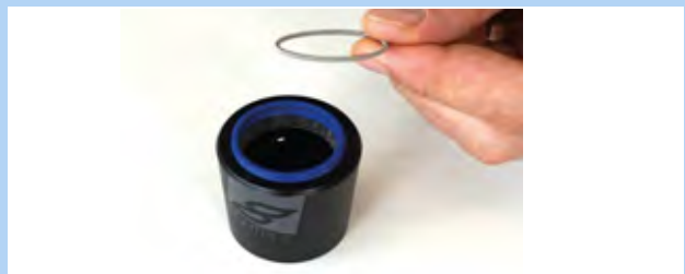
Figure 186: Removed spring washer
