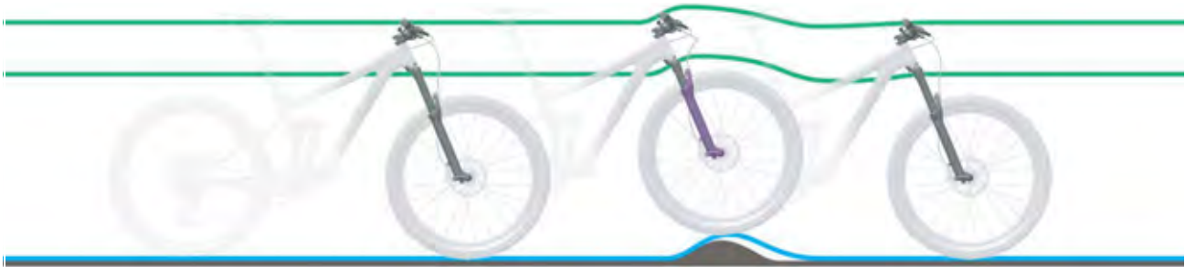
Figure 210: Excessively hard damping in the suspension fork on bumps
