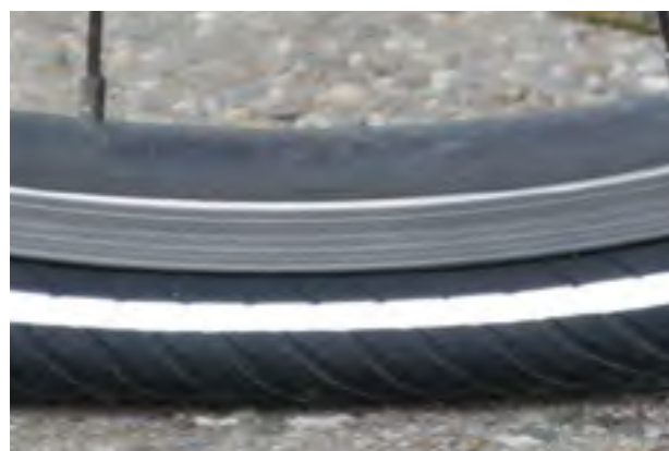
Figure 87: Much too little tyre pressure
